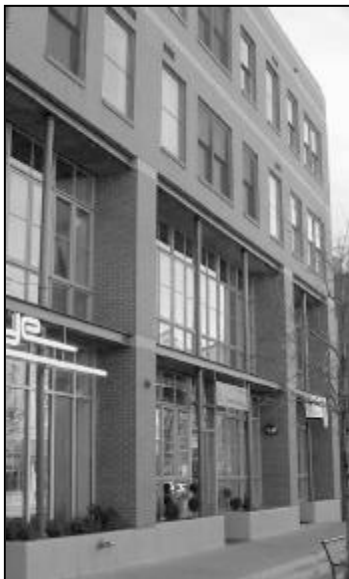
This building front has variations in its depth. A planter serves to define the front line at the sidewalk edge.
